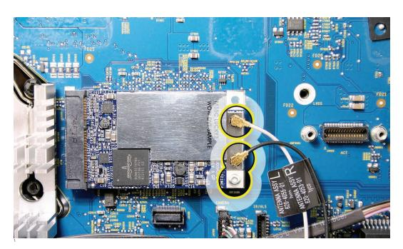
Holding the card by the edges, pull the AirPort Extreme card out of the slot.
